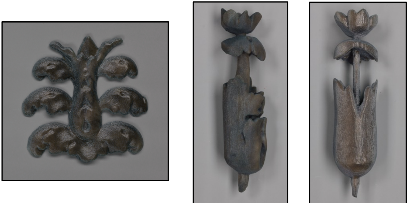
Figure 7. Examples of final 3D printed parts, before surface treatment and gilding.
