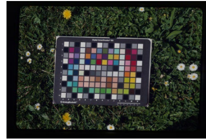
Figure 2: sRGB color rendering of the ColorChecker Digital SG shot on Kodachrome film, under daylight conditions.
