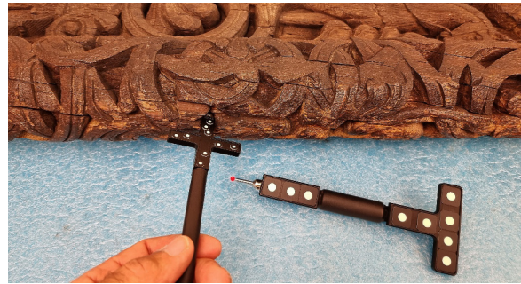
Figure 7. The GOM Touch Probe. I can mark the depth of cracks and plug holes in the project. This example is from the Hylestad portal. Photo Bjarte Aarseth
