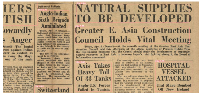
Figure 14. Localization error is significant in the large headline. The headline in the upper right corner was hardly identified by OCR software since some features were cropped by a bounding box.
