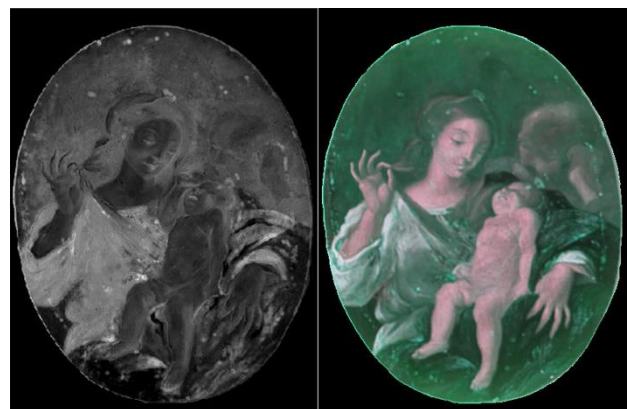
Figure 8. Concentration map for the EM 1 obtained with NMF (left). False RGB image of the restored painting with channels [695,980,905] nm (right).
