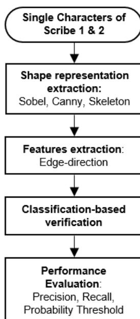
Figure 2. Flowchart of the proposed writer verification system.
