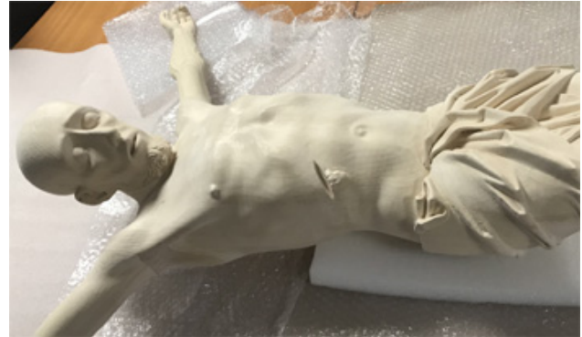
Figure 7. Copy of Christ sculpture made by CNC milling in linden wood (without any hand carving corrections), photo by E. Bunsch
