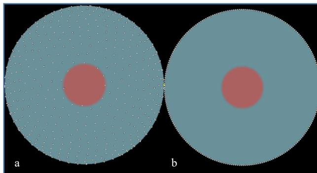
**Fig. 2:** Light positions for a) LDR acquisitions b) HDR acquisitions
