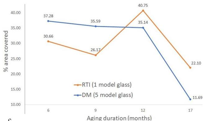
**Figure 5.** a) Standard deviation map of model glass aged for 9 months highlighting SN in yellowish-green colour ( $\approx 24 \times 21 \text{ mm}^2$ ) (examples indicated as inside red circles) b) Photomicrograph extracted from DM image of model glass aged for 9 months ( $\approx 5 \times 5 \text{ mm}^2$ ) highlighting SN (examples inside red circles) c) Graph showing temporal progression of percentage area covered by SN for model glass aged for different durations
