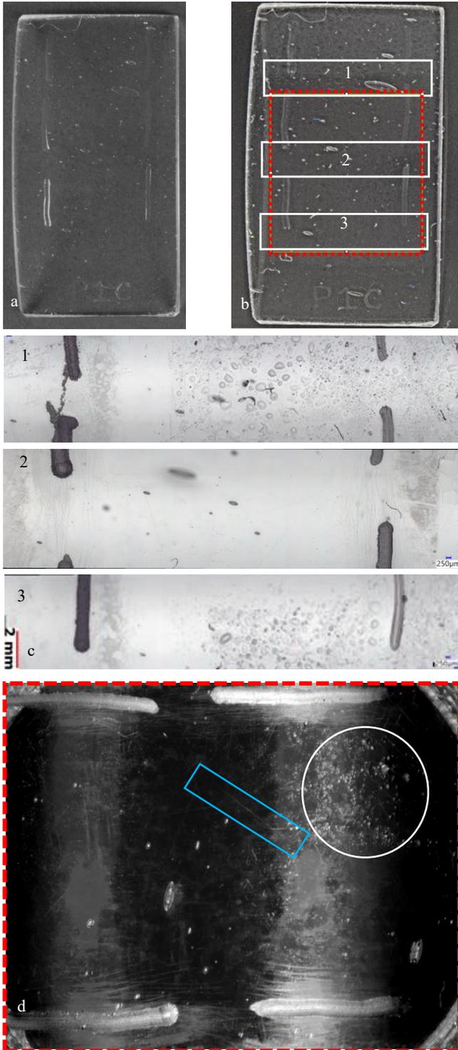
**Figure 3.** Visible light RGB photograph of model glass ( $\approx 50 \times 30 \text{ mm}^2$ ) aged for 9 months and wiped in the centre a) in diffused reflected light on black background b) in transmitted and cross-polarized light, showing the three DM narrow bands of acquisition (inside white rectangles) and one RTI acquisition region (inside dotted red rectangle) c) three narrow bands of model glass
