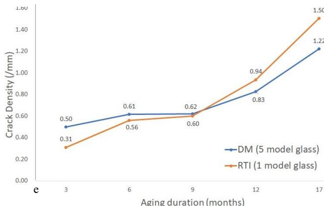
**Figure 4.** a) (Shannon) entropy map of model glass aged for 9 months along with the b) manual tracing of cracks ( $\approx 24 \times 21 \text{ mm}^2$ ) c) Photomicrograph extracted from DM image of model glass aged for 9 months ( $\approx 5 \times 5 \text{ mm}^2$ ) along with d) manual tracing of cracks e) Graph showing temporal progression of crack density for model glass aged for different durations
