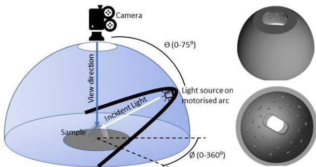
**Figure 1.** Schematic diagram of the RTI dome setup with matte black plastic background designed for reducing noise.
