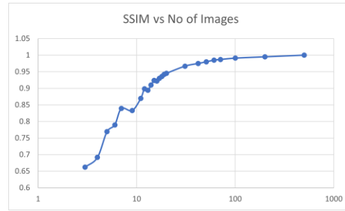
Figure 5. The normal map reconstruction converges after certain no of images in MLIC. This is performed on sculpture dataset.
