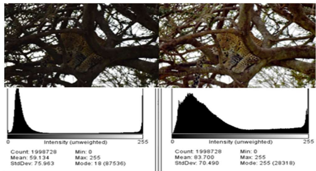
Figure 3. Contrast and Despeckling and Background Subtraction Yielded a 31% confidence improvement over the original image
