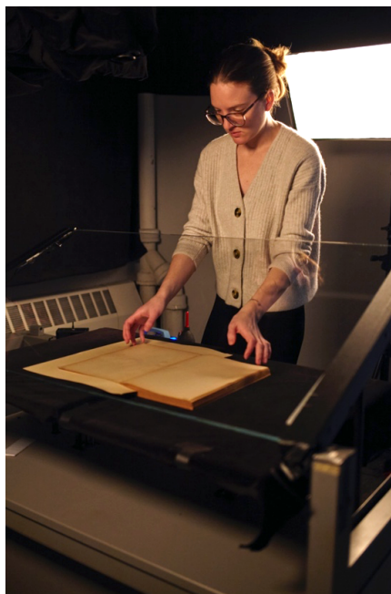
Figure 2. Photographer Sami Wright interleaves the notched page-tone background between the pages of a bound volume during imaging.
