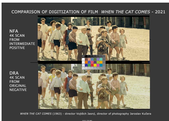
Figure 4 Comparison sampler 2 of digitized film “When the Cat Comes”, by director Vojtěch Jasný. Above, the NFA Final Master DCP made from Eastman Intermediate Positive; below, the DRA made from Eastman Original Negative. Scene with children walking in a square in the city of Telč.
