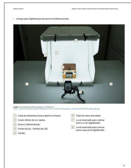
Figure 3. Workspace for three-dimensional items using the LED panels included in the studio box (page extracted from the Guidelines)
