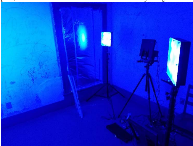
Figure 2. Multispectral imaging setup in Brandy Station Graffiti House with 100MP camera, filter and two narrowband light panels
