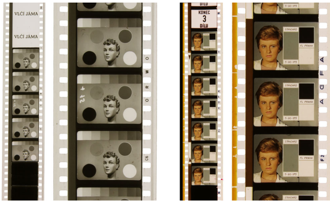
Figure 7 DRA Reference test patterns in the black-and-white ORWO positive print of the film The Wolf Pit and the AGFACOLOR colour print of When the Cat Comes . The grey reference patches are easily measured using specialized densitometers.
