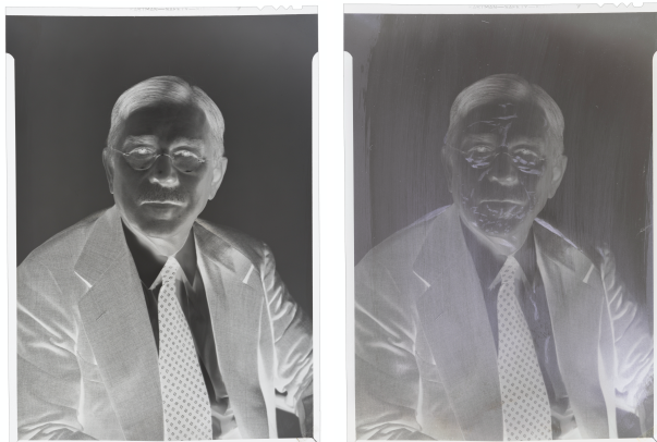
Figure 2. Example of one acetate negative with graphite retouching. Illuminated with both transmissive light (left) and specular light (right).
