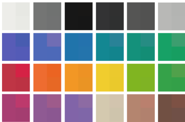
Figure 8. Color rendering visualization of the measured color (left half of each square), the color rendered from the RGB image (top right quarter of each square), and the color rendered from the 10-band image (bottom right quarter of each square).
