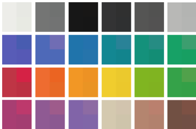
Figure 9. Color rendering visualization of the measured color (left half of each square), the color rendered from the RGB image (top right quarter of each square), and the color rendered from the 6-band combined image (bottom right quarter of each square).
