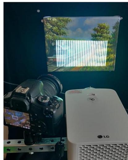
**Figure 3** A typical projector-camera rig for FPP.
