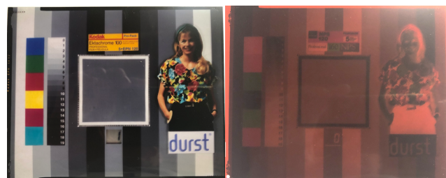
Figure 4. Example positive and negative film. The six patches along the left side were measured and used to evaluate the transmittance imaging system.
