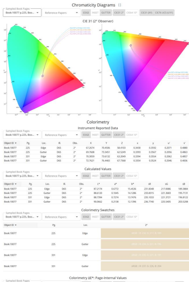
Figure 3. Some examples of the colorimetry data we could parse and compare across measurements on the same page and between different books, including the "same book" from different institutions. Again, all data is transformed from near "raw" in real time for each application.
