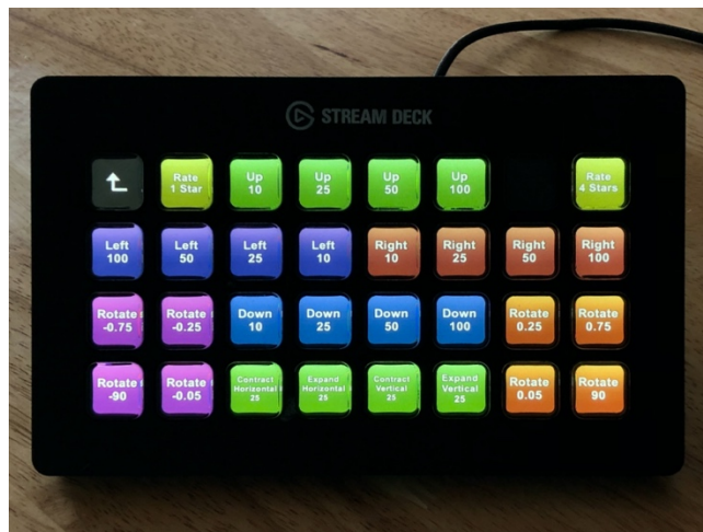
Figure 6. Stream Deck XL showing active buttons to adjust the size, location, and rotation of the crop box of the currently active image in Capture One Pro. Depending upon reproduction, it may be difficult to note that each type of action, such as “Up 25” and “Up 50”, share the same color buttons. Note buttons in the upper-left and right-hand corners to rate an image as “1 star” or “4 stars”.
