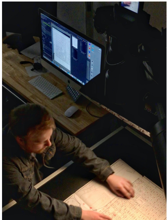
Figure 1. Andrew Coggins prepares a fragile map for digitization using a custom, camera-based capture station in the relocated Digital Production Lab at UT Libraries in late 2019. To his left is an Apple iMac running Phase One's Capture One Pro. This computer is tethered to and controls the camera. Part of Andrew's right hand is visible on the LCD-screen on the back of the camera in the upper-right hand corner of the image.
