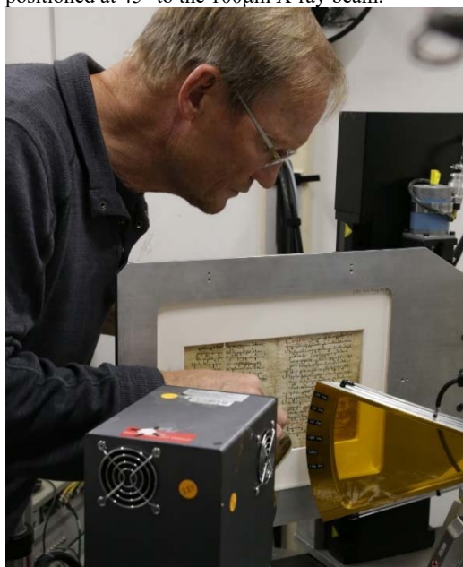
Figure 6. SSRL XRF scanning setup (x-ray beam from right) for the HMML Palimpsest being adjusted by Distinguished Staff Scientist Uwe Bergmann
