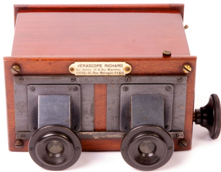
Figure 2. Inverter stereoscope or 'stereo redresseur' by Jules Richard, c. 1915
