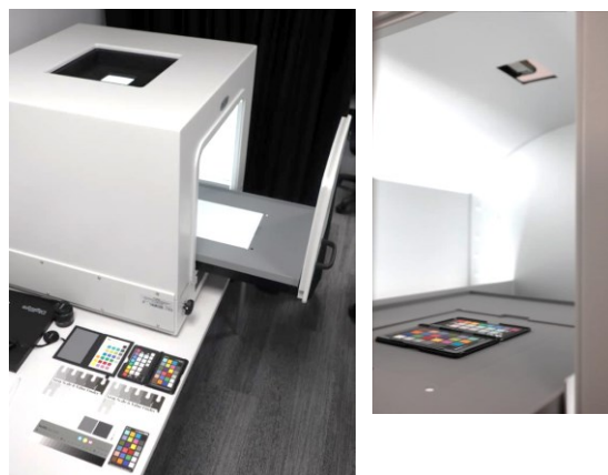
Figure 3. DigiEye by Verivide (left); Smartphone on top and imaging surface (right)
