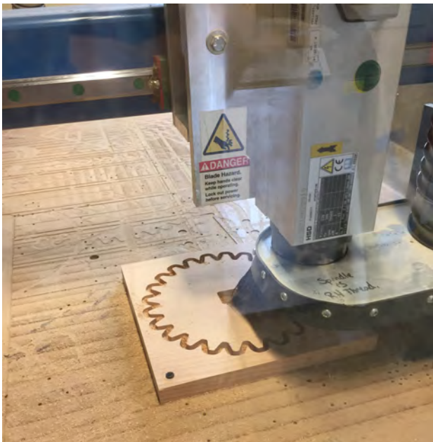
Figure 6. Computer numerical control routing of a gear for one of the Reading Wheels
