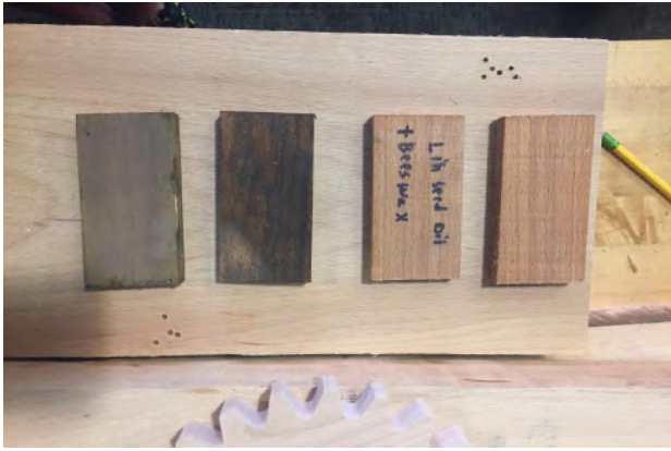
Figure 5. The team's experiment with various period-appropriate stains. From left to right: iron vinegar, iron vinegar and beeswax, linseed oil and linseed oil plus beeswax.
