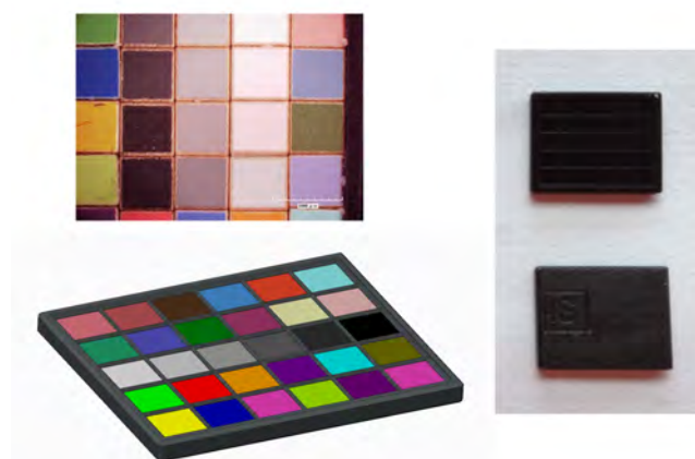
Figure 1. Original test target, top left, CAD model for prototype target, bottom left, 3D printed base plate, right, for a test target production process optimization project sponsored by Image Science Associates. 4
