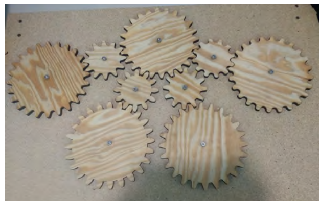
Figure 4. The team's prototypes of gear tooth profiles
