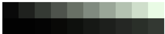
Figure 5. Simulation of twenty single full-field test images from nr. 17/1 to nr. 17/10 (black-to-white steps) and from nr. 18/1 to nr. 18/10 (black-to-dark steps) which are transformed for demonstration into sRGB color space with the adaptation to DCI-P3 white point.
