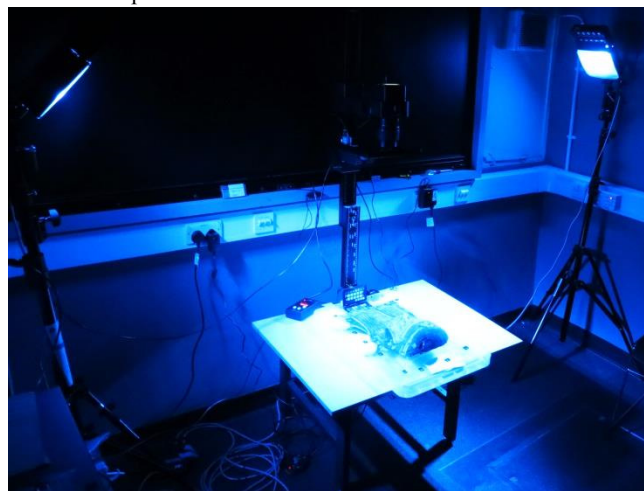
Figure 3. Multispectral Imaging system setup for UCL mummy mask imaging
