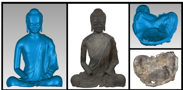
Figure 7 Final exterior 3D model and surface texture, Final interior merged 3D model (laser scan / photogrammetry) and interior surface texture
