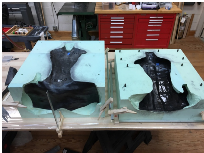
Figure 9 View of carbon fiber support elements in CNC milled molds
