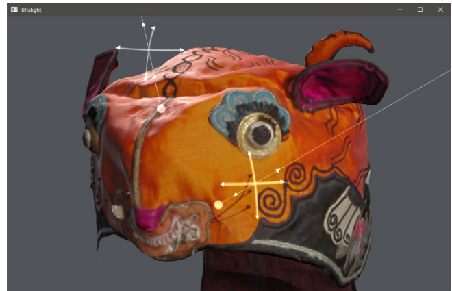
Figure 1. A child's tiger hat from the Minneapolis Institute of Art being rendered from 67 photographs according to the technique described in [2]. The manipulators drawn in white are a feature of IBRelight that allows the user to control the light sources illuminating the object.
