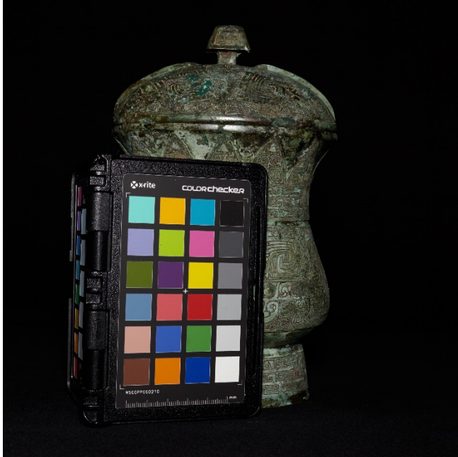
Figure 4. An example of a flash photograph containing an X-Rite Color Checker chart that can be used to calibrate the tone curve in the flash photographs used by IBRelight.
