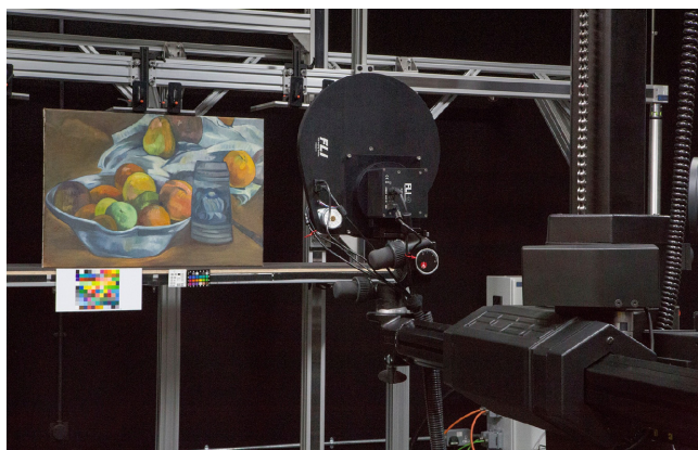
Figure 1. Multispectral imaging system being demonstrated in a workshop at the National Gallery, London.
