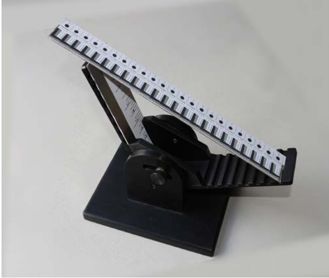
Figure 3: Example image capture setup with simple test chart, from Ref. 5.
