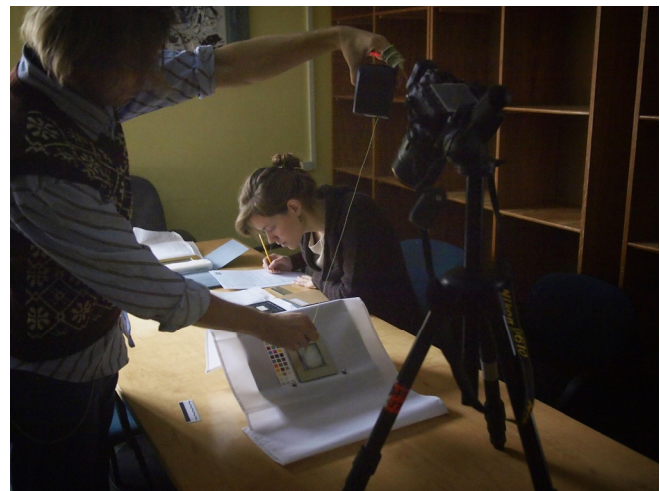
Figure 4. RTI capture in action. External flash is used as light source. Photo by Vahur Puik
