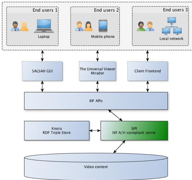
Figure 2. Architecture of Knora integrating SIPI as a IIIF-compliant media server capable of retrieving video content.
