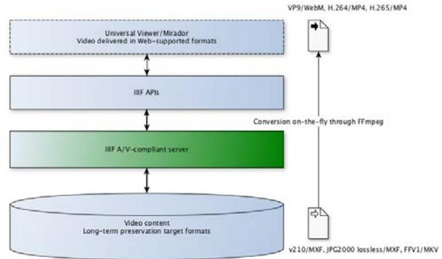
Figure 1. IIF and conversion on-the-fly with preferred destination formats for long-term preservation and for dissemination purposes
