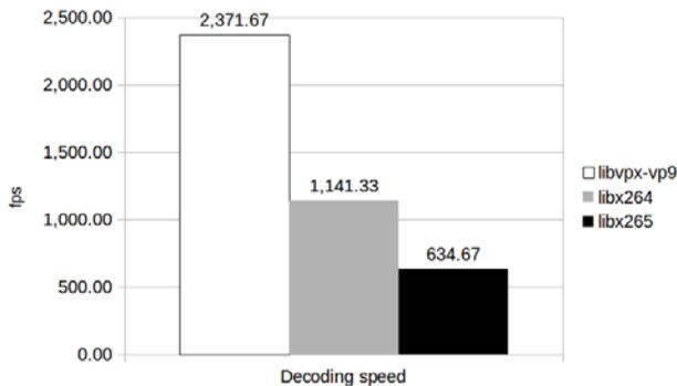
Figure 4. Average decoding speed (frames per second) between three libraries (libvpx-vp9, libx264, libx265) using FFmpeg on an off-the-shelf computer.
