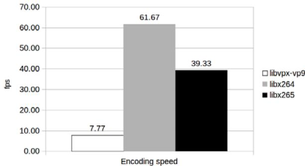
Figure 3. Average encoding speed (frames per second) between three libraries (libvpx-vp9, libx264, libx265) using FFmpeg on an off-the-shelf computer.
