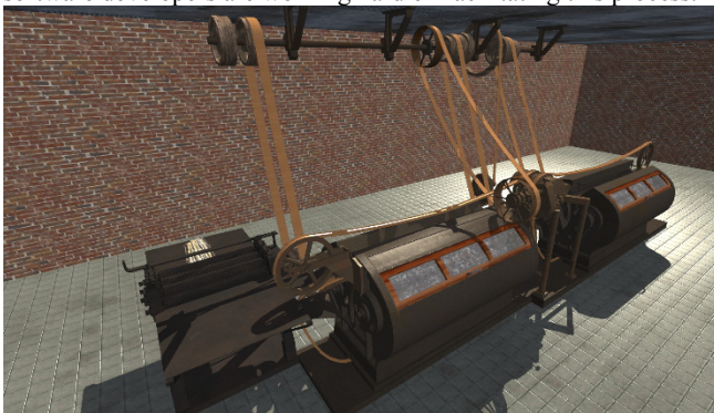
Figure 1 Low poly model generated from CAD model in visualization setup – Scutching Turbine
