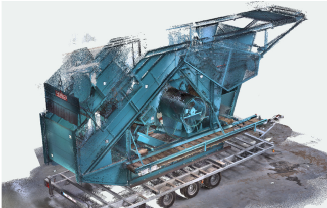
Figure 2 Point cloud made by handheld laser scanner – Hop Picking Machine
