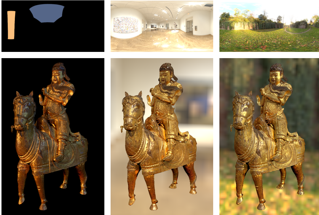
Figure 2. Image-based environment-mapping on a bronze statue of Kuan Yu. The environments used were, from left to right, a studio with color lights, a gallery at the Minneapolis Institute of Arts, and an outdoor scene.
