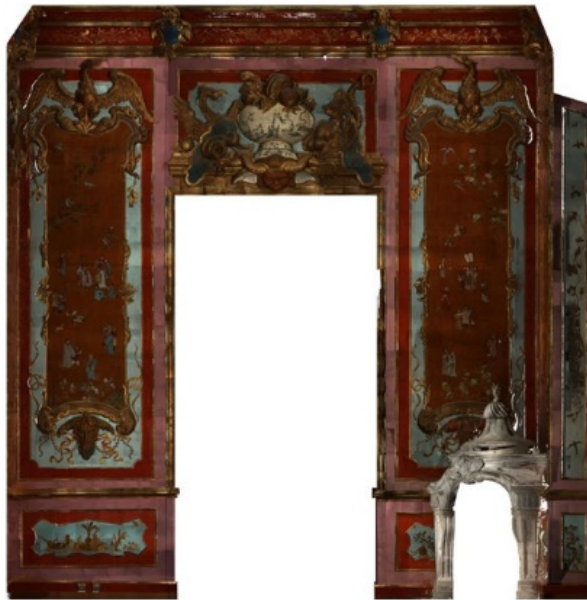
Figure 8. The King's Chinese Cabinet (Wilanów) – east wall. Dense cloud of points visualization (Massive software)
