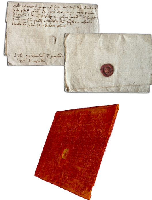
Figure 3: 1351 Venetian testament. Top: visible images of the recto and verso of the document. Bottom: 3D tomographic reconstruction with writings on the recto clearly visible.
