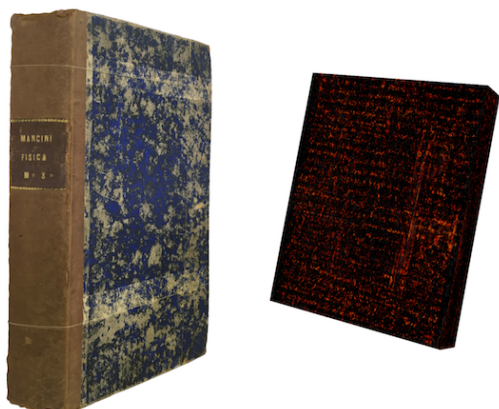
Figure 5: The 18 th century physics book. On the left: 3D reconstruction with visible light. On the right: a sectional view of the x-ray tomography reconstruction, where all the writings from the inside are visible.
