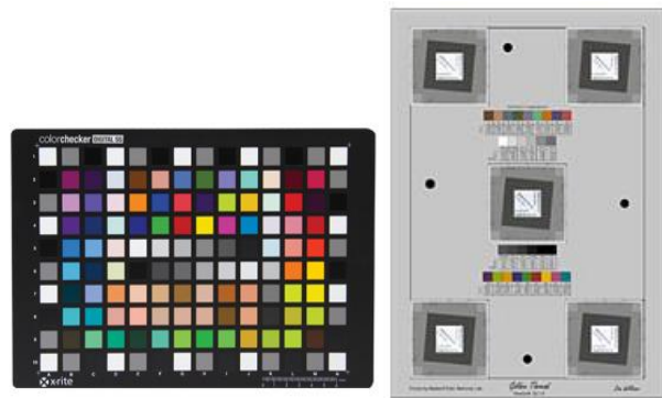
Figure 1. Examples of targets for device color accuracy assessment. Left: ColorChecker SG chart; Right: GoldenThread TM target.
