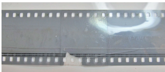
Example of physically damaged 35mm optical film sound track negative from figure 1, after repair.
