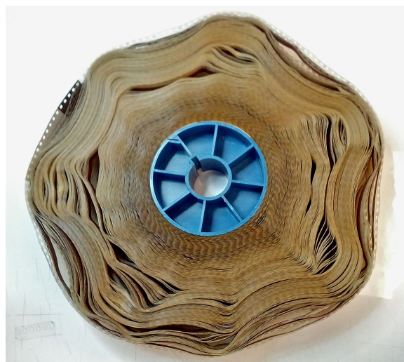
Severely dry and brittle 35mm magnetic film reel in need of hydration.
