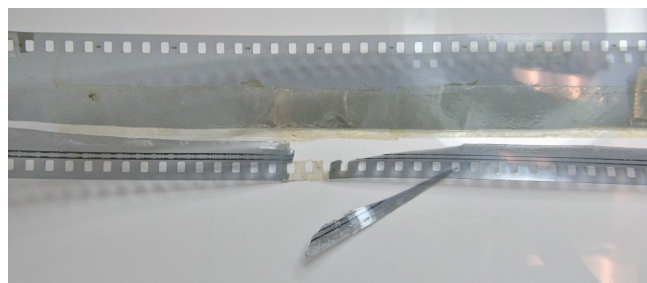
Example of physically damaged 35mm optical film sound track negative before repair.
