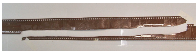
Example of physically damaged 35mm magnetic film sound track before repair.
