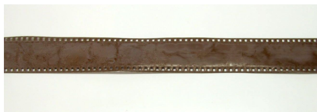
35mm magnetic film with heavy plasticizer build-up, before alcohol treatment.
