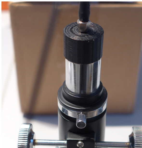
Figure 4. Custom eyepiece with fiber inserted in metaloscope.
