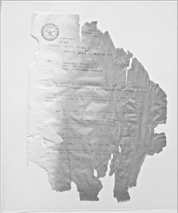
Figure 13: The same document in Figure 12, but infrared image. Tones that define the surface features compete with text readability. The best lighting is soft enough to evenly light the surface, but not so soft as to create glare on polyester film surface.
