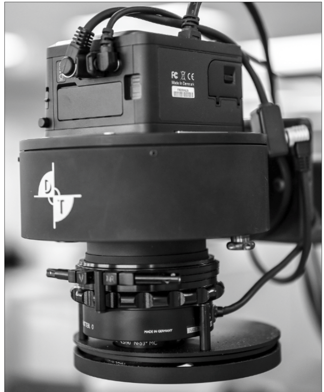
Figure 9: The DT Multispectra camera with a 60 megapixel camera back. Focus locks and filter turret make it ideal for adapting shot types in consecutive shots.
