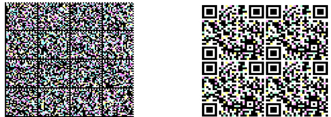
Figure 3: Demonstration of barcode with two channels. The black and rest-as-white will read with an off-the-shelf reader, the right Data Matrix will display an abstract and the left QR-Code displays a test message.
