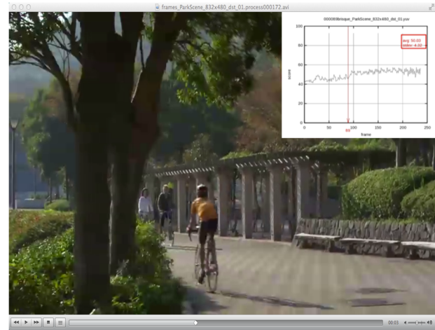
Figure 6. Screenshot from the visual diagnostic tool showing the current frame along with its score and the scores for all other frames.
