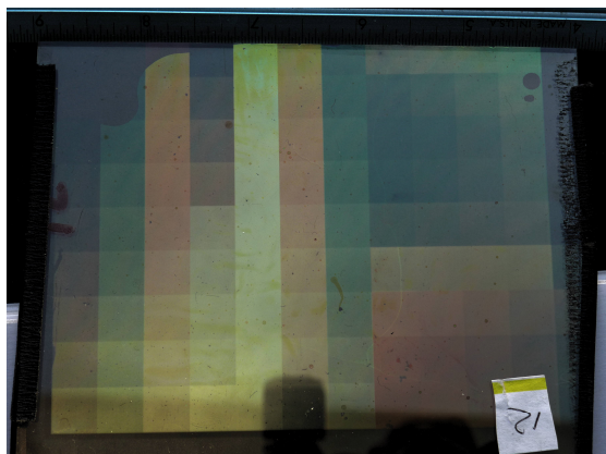
Figure 1. Plate #12 showing multiple irradiance levels for each color of an IT8 transparency exposed with CF non-coherent light and constructed with a mercury bath for a reflector. Photographed as irradiated by skylight
