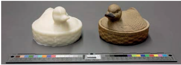
Figure 5. 3D print from photogrammetry-produced STL file (ABS print by Thomas Mealy from virtual model by author).
