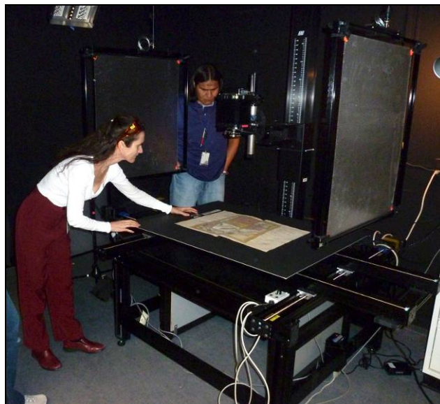
Figure 1. Spectral Imaging System at the Library of Congress
