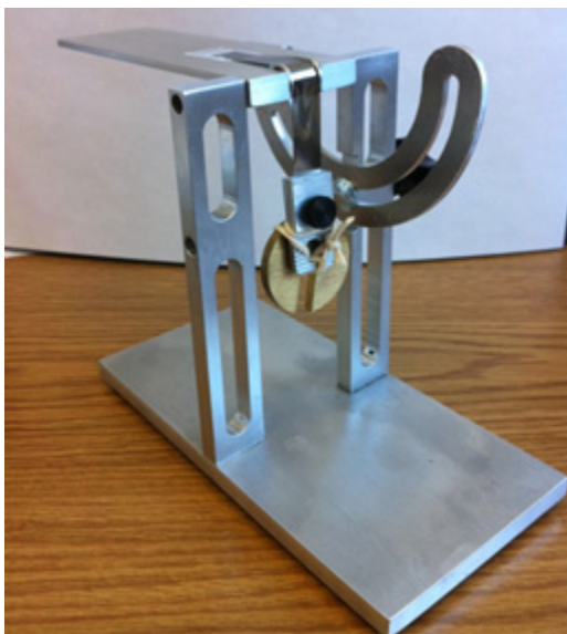
Figure 9: The weight stand test fixture, over which the tape is draped and tensioned, then moved back and forth.
