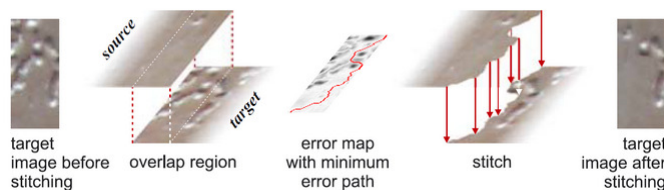
Figure 1: Outline of steps used in current image stitching software (from Ref. 2)
