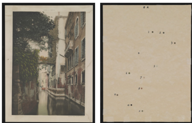
Figure 3. Sample print A without and with its mask showing the 11 selected color areas or regions of interest.
