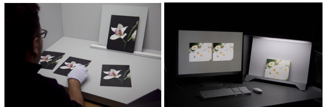
Figure 3. The hardcopy (left) and softcopy (right) experimental setups
