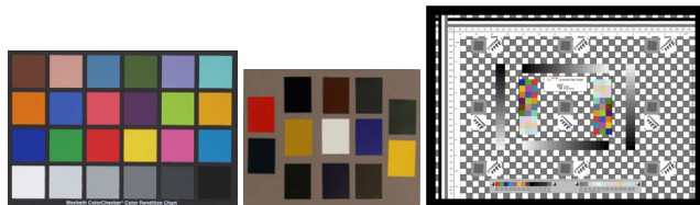
Figure 2. The targets for the Current Practices in Fine Art Reproduction project, from left: Macbeth Color Checker, paint patch target, Universal Test Target®
